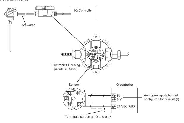
Note that if connecting to an IQ22x controller, do not connect to C (+24V), instead connect to AUX+ (+24V).
