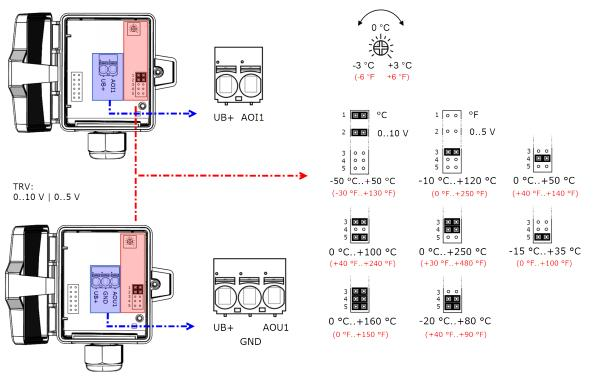
fig. (Measuring range and offset adjustment, default settings: -50 °C..+50 °C | 0 K)
