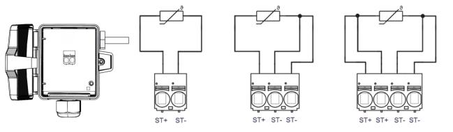
fig. (terminal assignment passive sensor)
