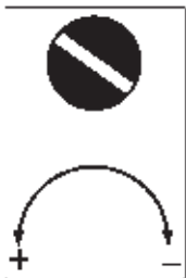
Direction of action of setting spindle
