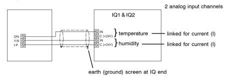
Note that when connecting to IQ3, in order to provide sufficient supply current to the sensor, the sensor I-P terminal must be connected to **both** channels' 24 V terminals.
