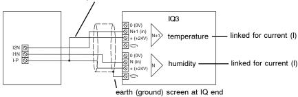
Note that in order to maintain the HT/S/2% temperature sensor accuracy, the temperature sensor should only be used if the humidity sensor is also used.
