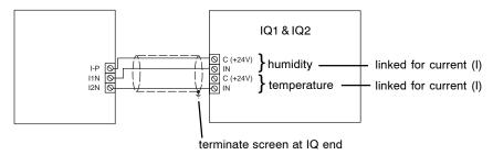
Note that when connecting to IQ3, in order to provide sufficient supply current to the sensor, the sensor I-P terminal must be connected to **both** channels' 24 V terminals.
