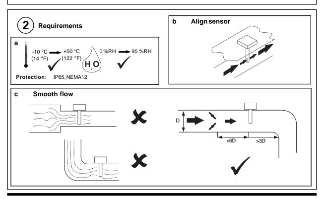
AV/D Duct Air Velocity Sensor Installation Instructions TG200504 Issue 3, 22/12/2010
